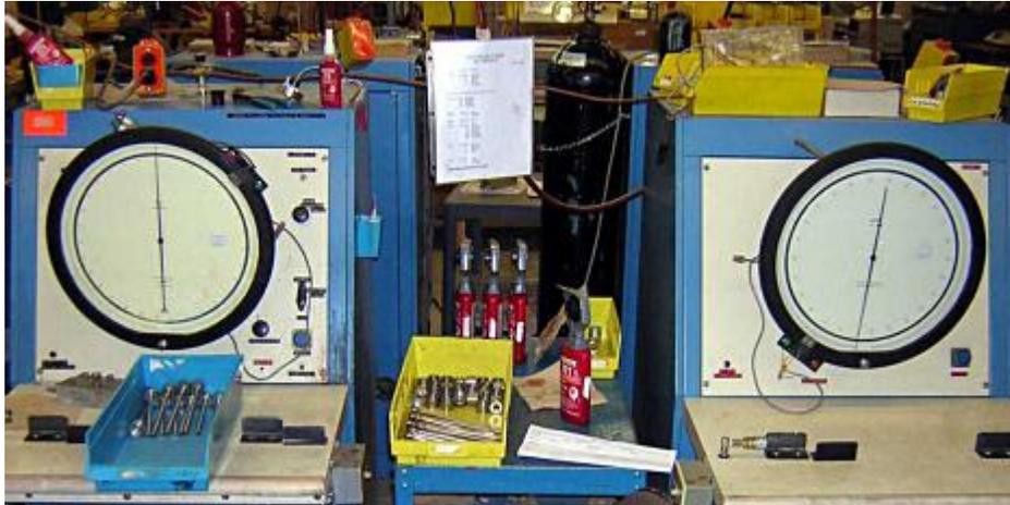
Figure 1. A group of calibration stands, which allow operators to install the set points into the pressure or vacuum switches
