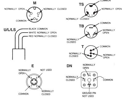
\*Vacuum Switches: Normally Open & Normally Closed are reversed
